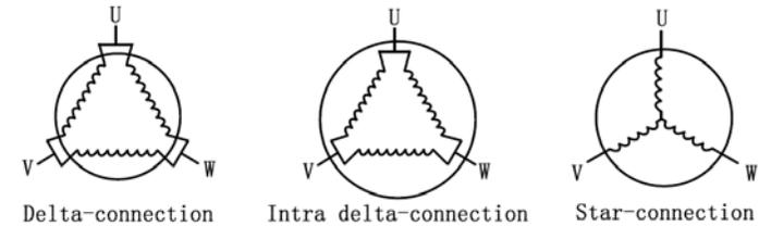
Figure 5: Motor connections
