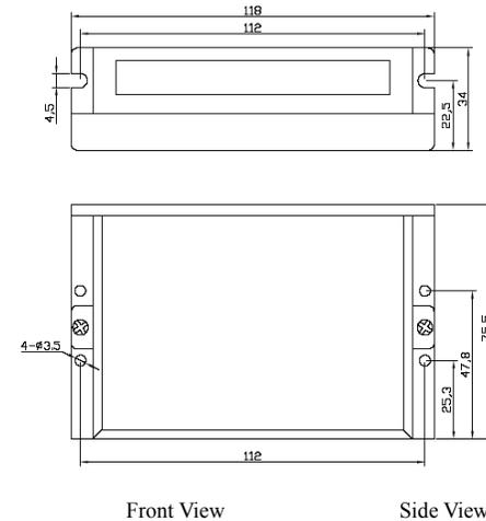
Figure 1: Mechanical Specifications
